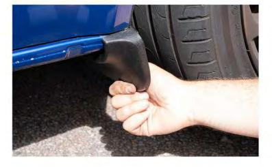
Secure your front mudflaps by driving the screws into the plastic wheel arch lining.
