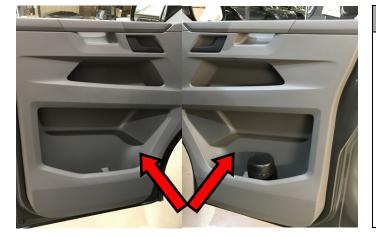
Remove the Driver's and Passenger's front door trims.
