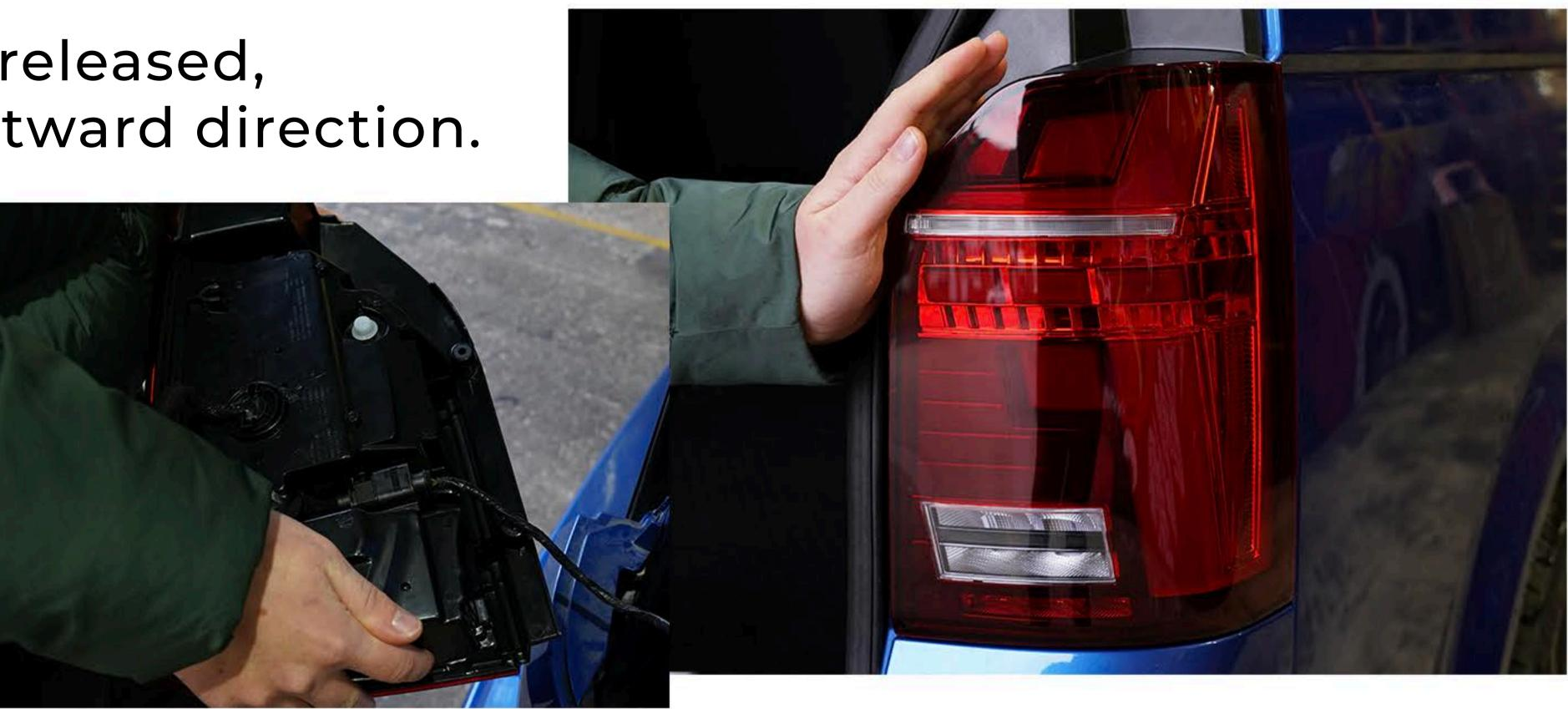
Make sure to keep hold of the light as it will still be connected to the electrics.
