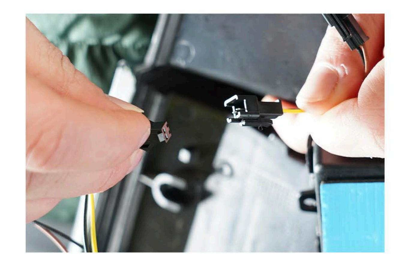
If you have fitted one resistor and the lights aren't working, we recommend on fitting your second resistor.
