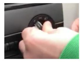
Unplug the connector on the back of the switch.
